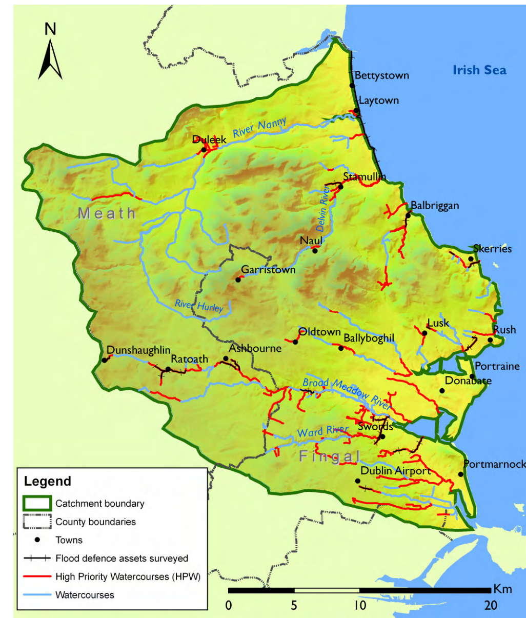
Map of the Fingal East Meath study area showing watercourses, HPWs and flood defence assets surveyed to date.
